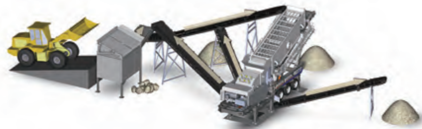
篦条料仓--快速实现多种破碎筛分工艺模式的转换 Grid hopper - quickly achieve switching among various crushing and screening process models
